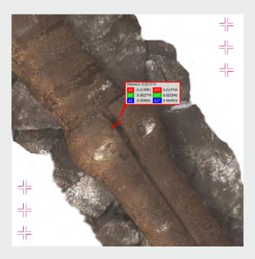
measurements of free-span, distance from the bell mouth into burial, gaps manifesting on CPS half shells, and much more from the comfort of their office. From one single scene that can be viewed on any device, anywhere in the world via Vaantage, users have a complete overview of the problem at hand, together with the information needed to start discussing solutions and inform potential remediation techniques such as underpinning or stabilisation by rock bag placement.
