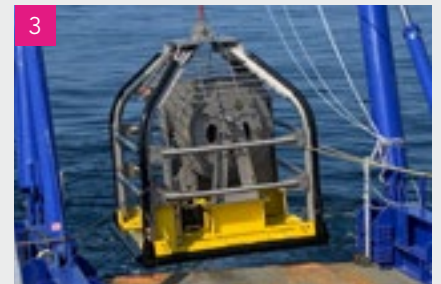
3 CPT launch for reliable, versatile and efficient sampling of in-situ soil conditions.
