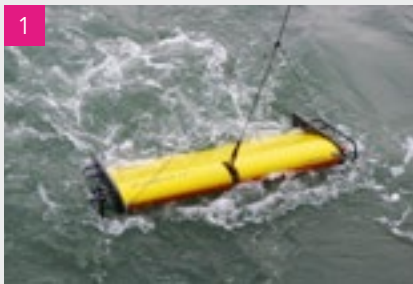
1 Equipped to deploy towed sensors such as SSS, ROTV or 2D-UHR.
