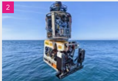
2 Work-Class ROV, enabling detailed surveys of areas of interest such as inspection of cable crossings, or archaeological surveys. Deployment with Pilot Assist/RPL following capability.
