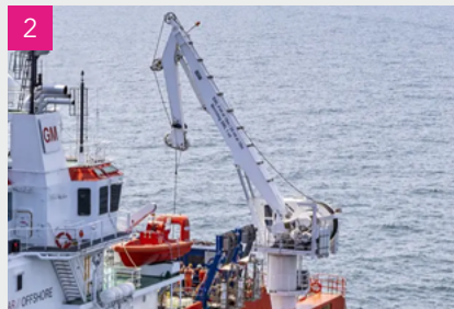
2 Active Heave Compensated - Subsea Crane, assures precision and safety during critical operations.
