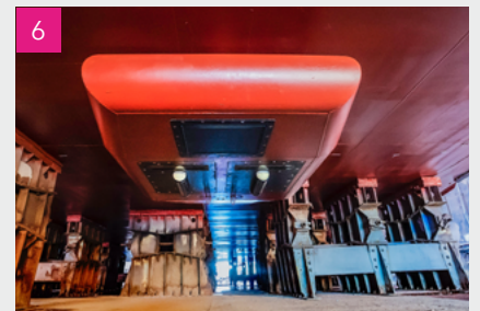
6 Hull mounted survey sensors enable high quality, repeatable MBES (2x R2sonic 2026) and SBP (1x Innomar Medium-100) data collection.
