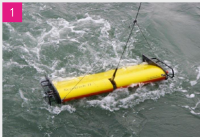
1 Equipped to deploy towed sensors such as SSS, ROTV or 2D-UHR.
