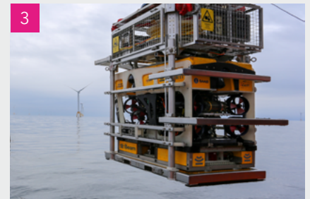
3 Work-Class ROV, enabling detailed surveys of areas of interest such as inspection of cable crossings, or archaeological surveys. Deployment with Pilot Assist/RPL following capability.
